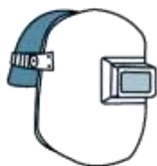
Face shield detached for a safety helmet, stationary window
