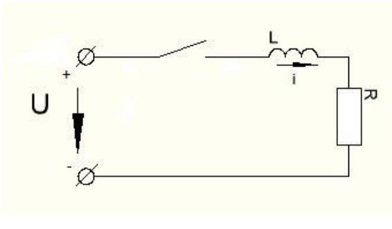
$$\begin{aligned} 1. \quad & i = 0 \\ 2. \quad & i = \frac{U}{R} e^{-\frac{R}{L}t} \\ 3. \quad & i = \frac{U}{R} - \frac{U}{R} e^{-\frac{R}{L}t} \\ 4. \quad & i = -\frac{U}{R} e^{-\frac{R}{L}t} \end{aligned}$$
