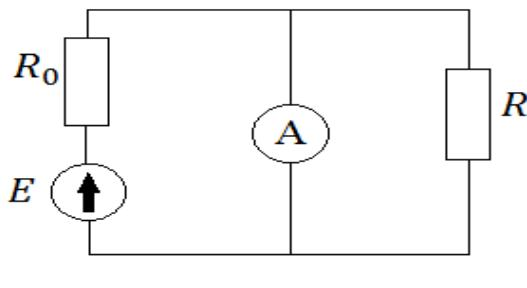
$$\begin{aligned} 1. I &= \frac{E}{R_0+R} \\ 2. I &= \frac{E}{R_0} \\ 3. I &= 0 \\ 4. I &= \frac{E}{R} \end{aligned}$$
