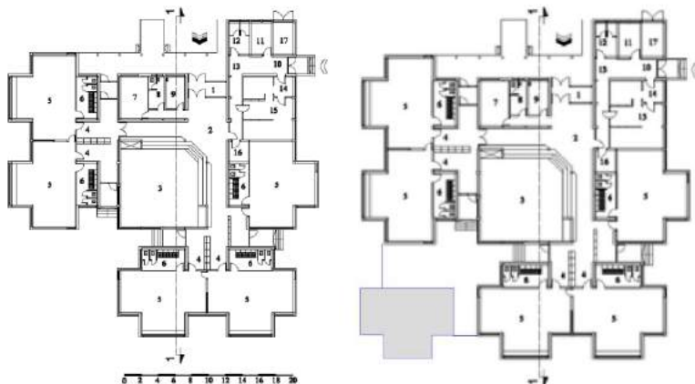
Fig. 5. Kindergarten "Pčelica", Vranje, Serbia, architect S. Dimitrijević, existing state and possible extending of capacity
