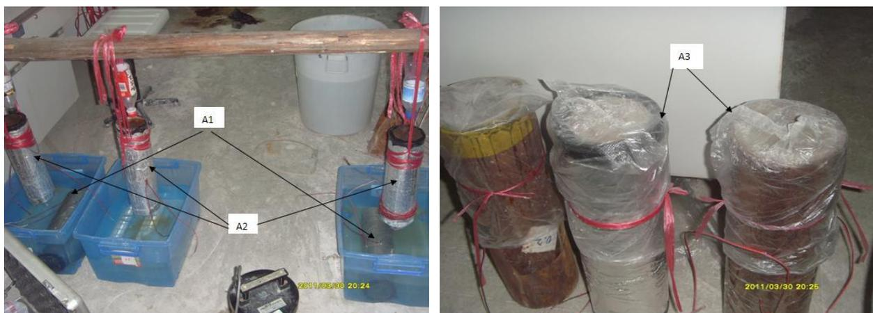
Fig. 8. Corrosion of samples of A1, A2 and A3 series
