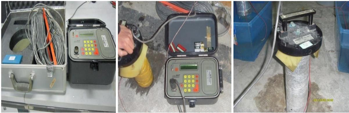
Fig. 9. Apparatus (Gecor6) of corrosion current densities
